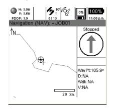
The navigation screen is framed to provide the map display along with active navigational controls and text. The framed control panel contains a directional guidance arrow, and text fields providing:
